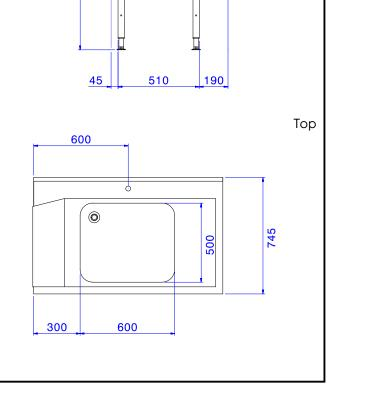
Handling System for Hood type Pre-wash Table with 600x500 Bowl Right to Left, 1200mm
